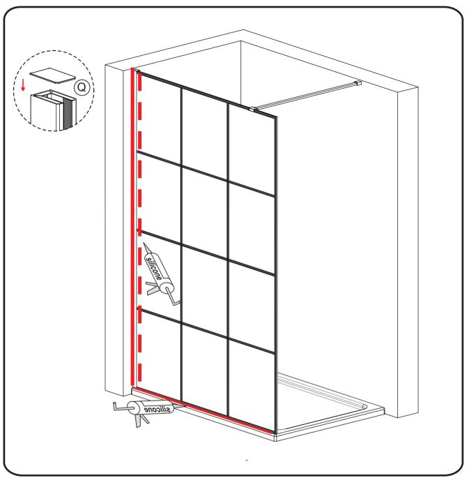
Step 12. Fit the top cap onto the wall profile (Diagram Q)
