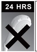
DO NOT USE THE ENCLOSURE FOR 24 HOURS AFTER SEALING
